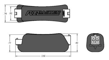
Figure 4. RFID Interface Module
