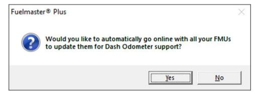
If **No** is selected, focus returns to the Dash Odometer Data Set dialog. Site Configuration updates and Online sessions verify the Dash Odometer Data Set files existence and version and, when necessary, transfer appropriate Dash Odometer Data Set files to the FMUs.
