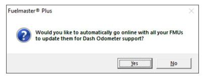
If Yes is selected, an Online session is initiated and the three Dash Odometer Data Set files are transferred to each FMU and placed on the compact flash card in the "aim\_dash\_odom" folder.
