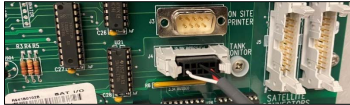
Figure 2 Cable to Sat I/O Connection
