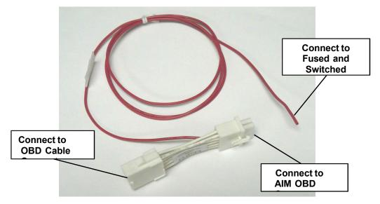
The 941B0509 AIM Switched Power OBD Adapter will only fix problems generated by a power drain through the AIM module. The Sleep Test and Current Draw Test will determine if installation of the adapter is necessary to resolve battery drain problems. Both these tests should be performed before installing the adapter.
