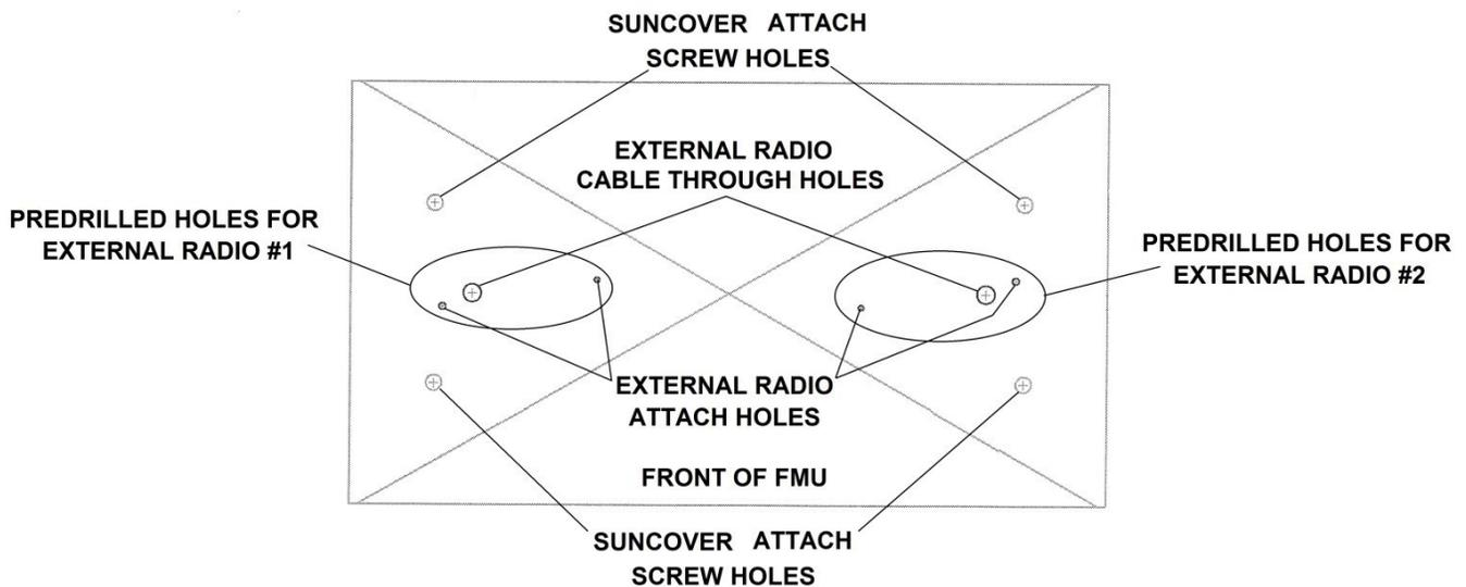
Figure 6. FMU Suncover Predrilled for External Radios
