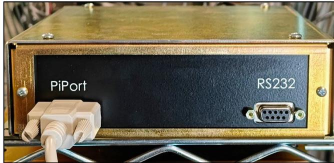
3. Connect the other end of the serial cable to either Pi Port 1 or Pi Port 2 of the Omega JR, depending on the addressing of the dispenser. Pi Port 1 connects to addresses 1-16, while Pi Port 2 connects to addresses 17-32.
