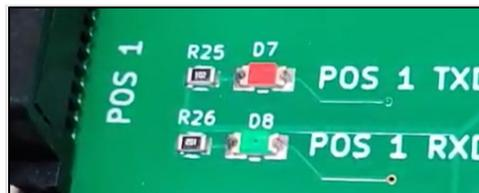
Finally, when connected to a dispenser, the Bank 1 lights should show activity. These lights are to the right of and below the HB light. The red TXD and the green RXD should blink, but the speed at which they show activity can vary from dispenser to dispenser. The cream CTRL light should be lit if the Omega JR is powered up.
