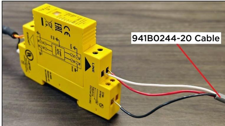
**NOTE** The 941B0244-20 is an RS-232 cable, normally limited to 50 feet. This may be exceeded by increasing the conductor size and cable quality. If in doubt, test the connection before pulling the cable through conduit.
