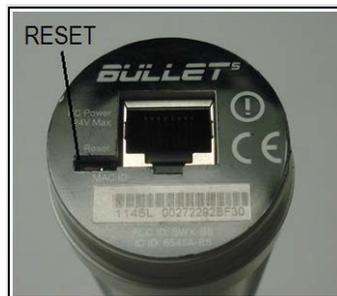
Figure 15 Bullet Reset Switch
