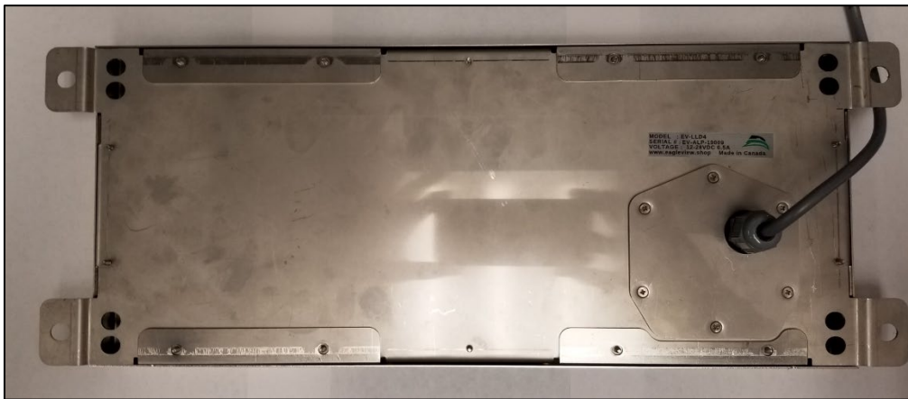
Figure 2. Interface Cable attached to back of Single Line Display
