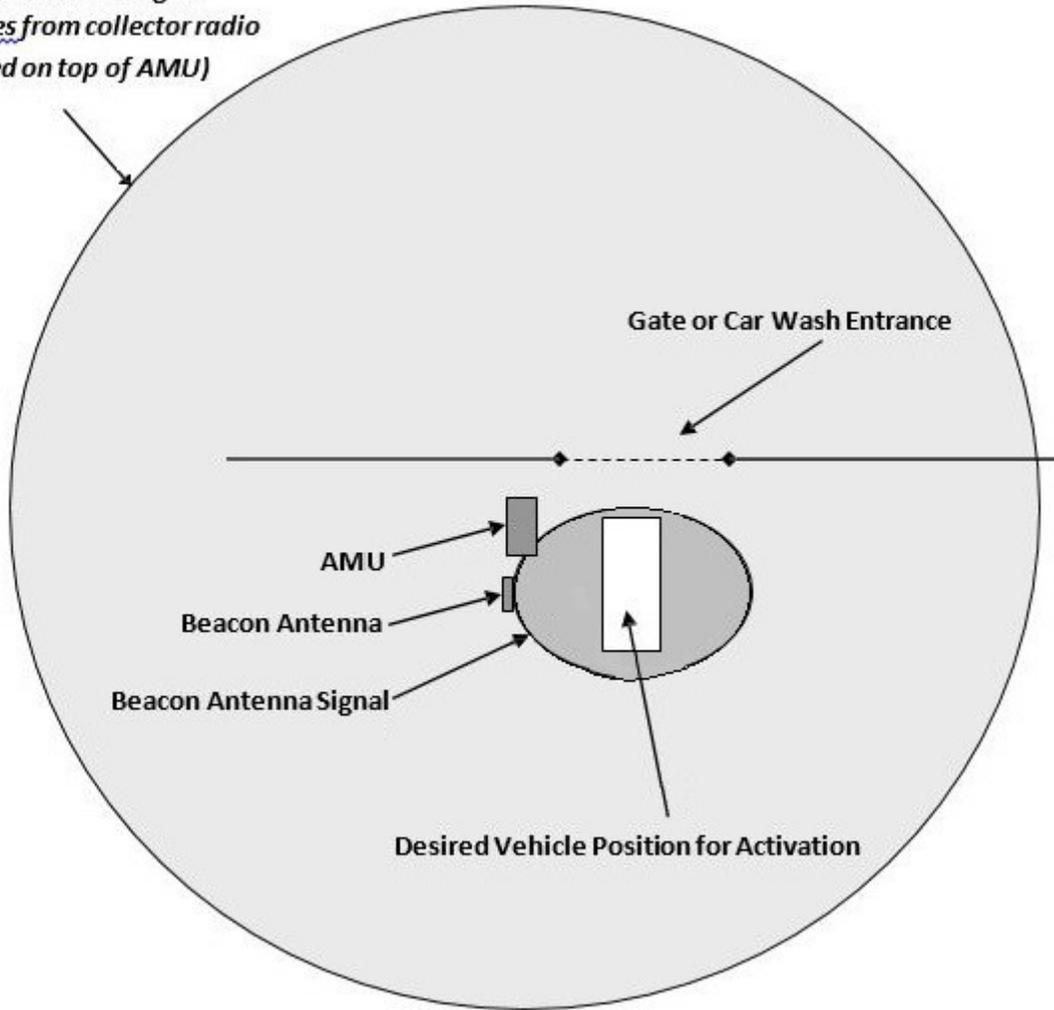
Figure 4. Overhead View of Control from One Direction Only
