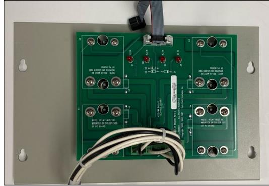
**Figure 26 Installing the New Relay Board**
