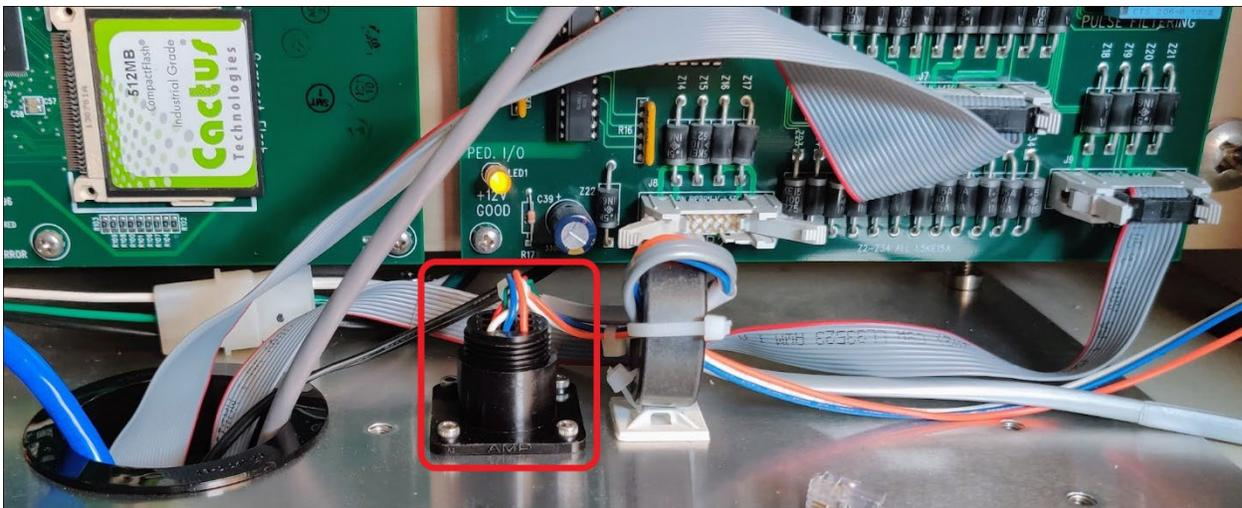
Figure 4 Bulkhead Connector
