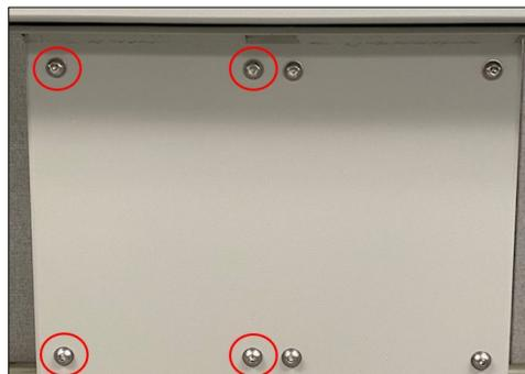
Figure 13 The Relay Board Screws
