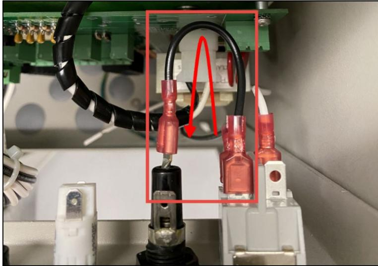
Figure 8 Connecting the Black (Hot) Wire
