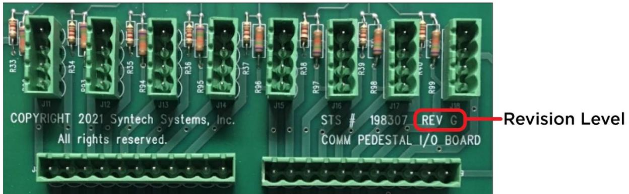
Figure 19 Ped I/O Revision Level
