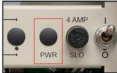
Figure 10 The Power LED Plug
