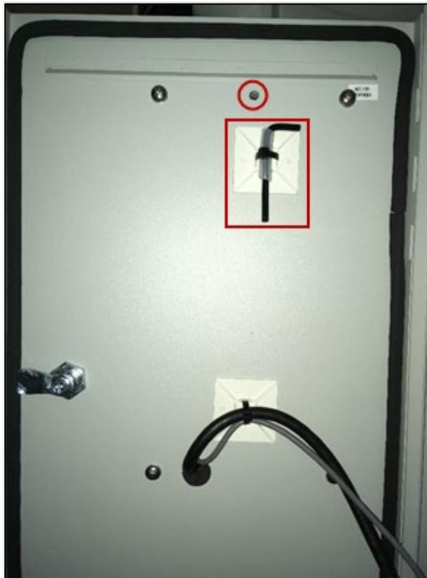
4. Loosen the cover (hinged at the bottom) and pull the top down to expose the backplate assembly.
