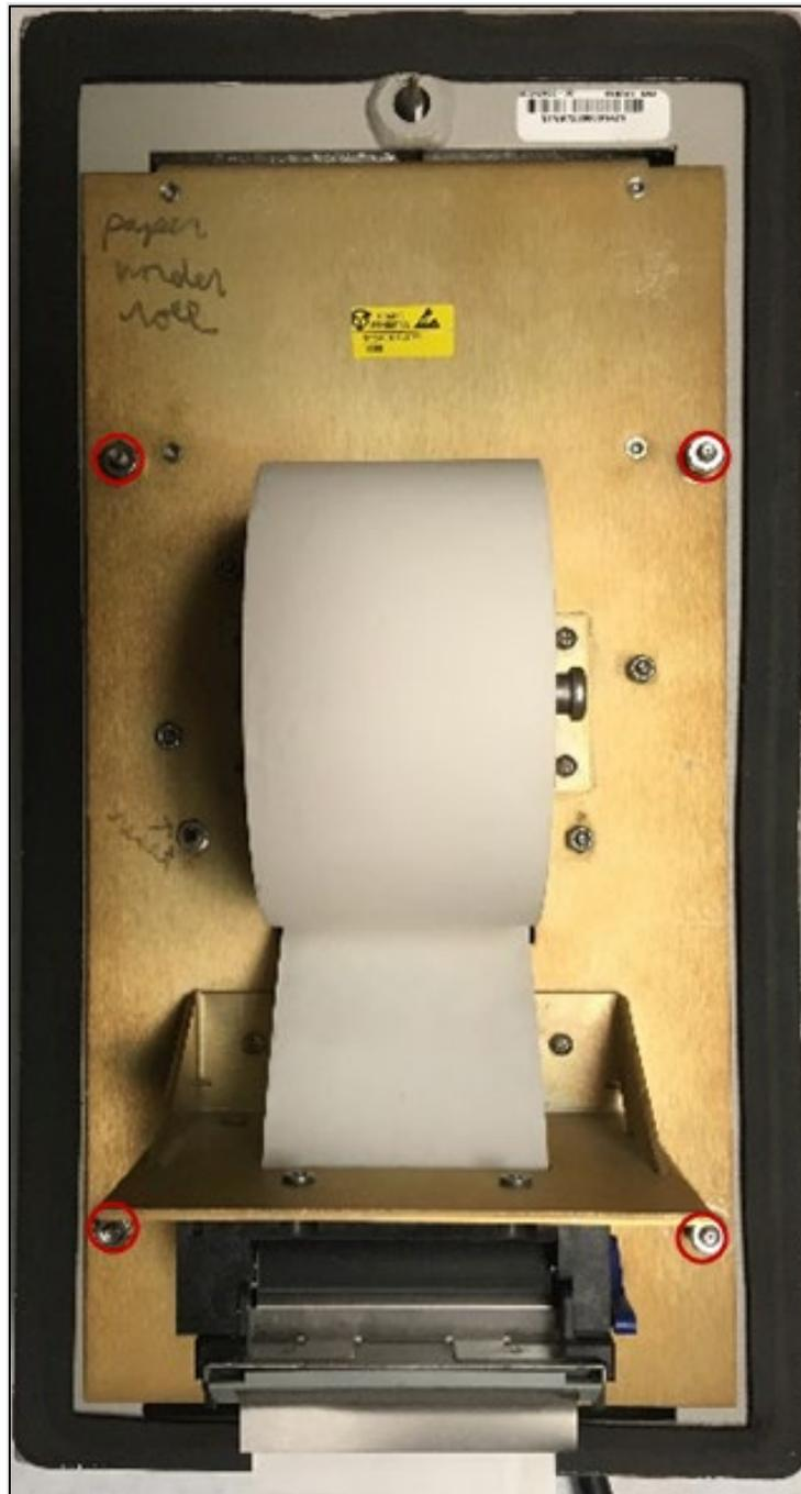
6. Carefully remove the backplate assembly from the housing.
