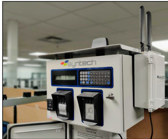
Figure 1 The MDU with antennas adhered to the right side of the FuelMaster Unit (FMU)
