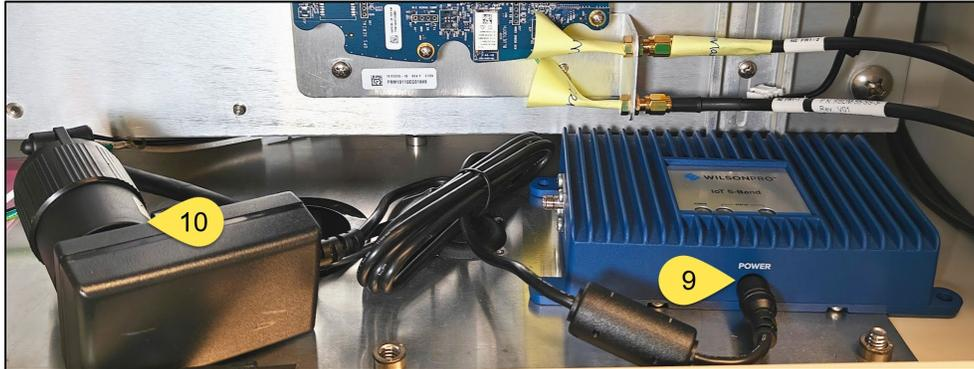
11. Disconnect the existing external Primary Antenna cable from the EAPro's Primary Antenna lead.
