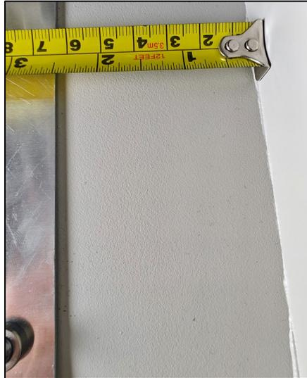
2. Drill out two ¼-inch holes - large enough to insert the threaded portion of the bulkhead connector but not the whole connector.
