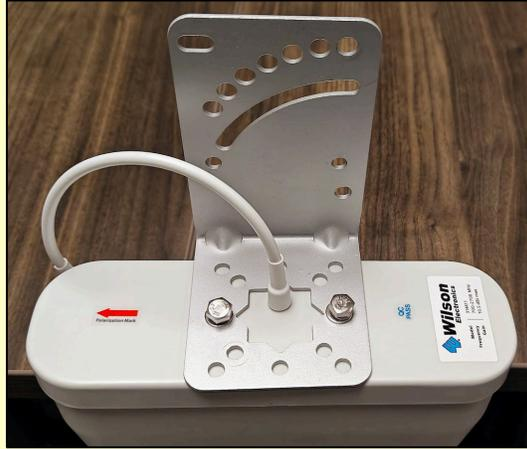
1. Unscrew the 2 bolts, as well as the associated washers, holding the L-Bracket to the antenna.
