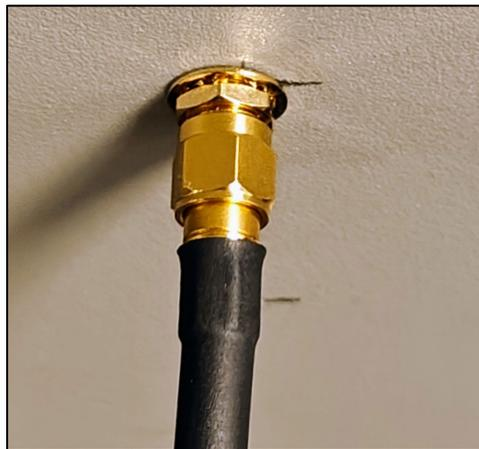
7. Turn the FMU on and test the connection. The final product inside the FMU head should appear similar to the below picture.
