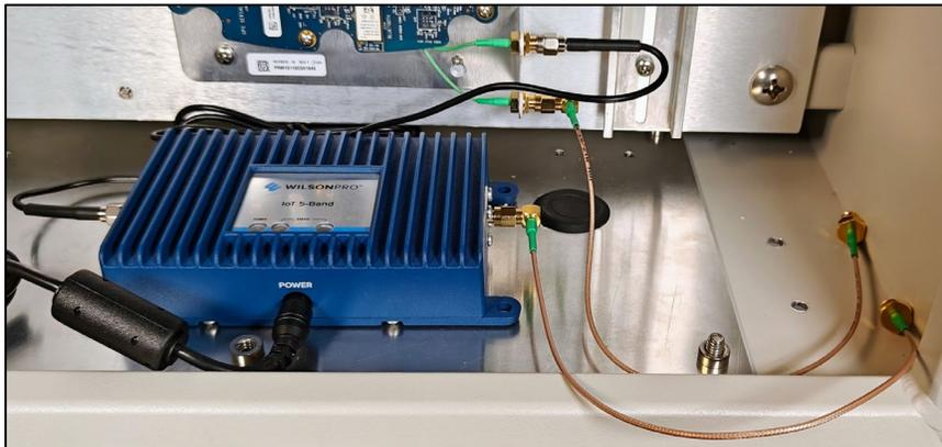
3. Unscrew the nut from each of the bulkhead cables.
