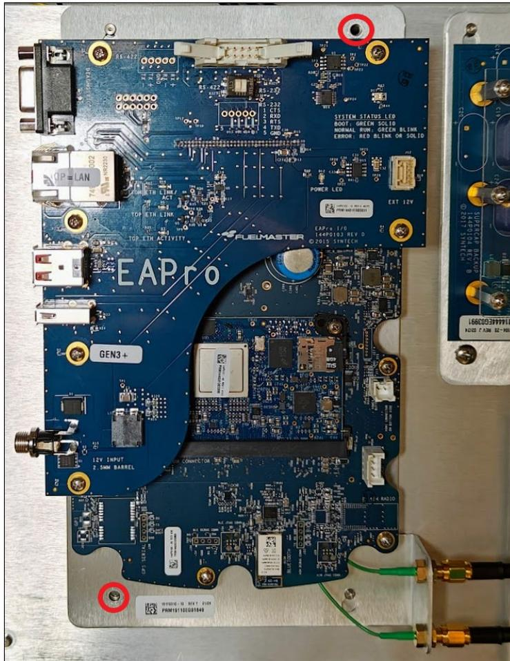
4. Find the X1 and X2 connections (these may be upside-down, as seen below) where the antenna leads connect to the back of the EAPro.
