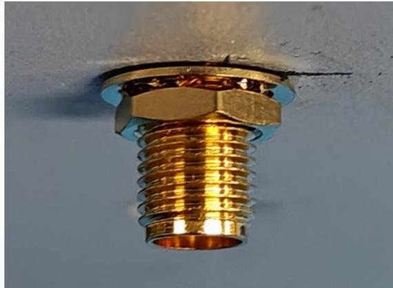
6. Attach the cables from the external antennas to the bulkhead connectors on the bottom of the FMU head.
